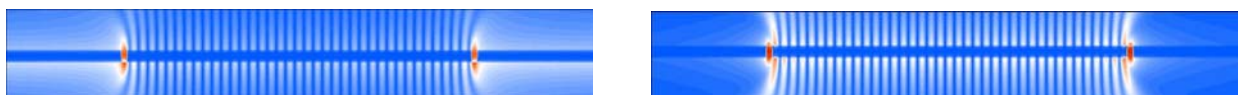
Fig. 1. The amplitude of the scattered magnetic field when a metal plate with two parallel slits of widths equal to a quarter of the wavelength, is illuminated by a p-polarized plane wave from the top. At the left the distance between the slits is such that a minimum of transmission occurs, at the right the distance gives a maximum.
